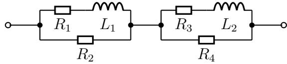
$$R_1 = 100 \Omega \quad R_2 = 200 \Omega \quad R_3 = 200 \Omega \\ R_4 = 100 \Omega \quad L_1 = 0,1 \text{ H} \quad L_2 = 0,1 \text{ H} \quad \omega = 1000 \text{ s}^{-1}$$
