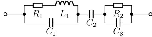
$$R_1 = 100 \Omega \quad R_2 = 200 \Omega \quad L_1 = 200 \text{ mH} \quad C_1 = 2 \mu\text{F} \quad C_2 = 10 \mu\text{F} \quad C_3 = 2 \mu\text{F} \\ \omega = 1000 \text{ s}^{-1}$$
