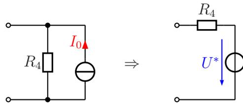
$$U^* = R_4 \cdot I_0 = 2 \text{ k}\Omega \cdot 10 \text{ mA} = 20 \text{ V}$$
