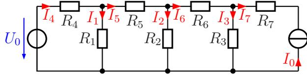
$$U_0 = 12 \text{ V} \quad I_0 = 20 \text{ mA} \quad R_1 = 1,4 \text{ k}\Omega \quad R_2 = 4 \text{ k}\Omega \quad R_3 = 1 \text{ k}\Omega \\ R_4 = 1,25 \text{ k}\Omega \quad R_5 = 1 \text{ k}\Omega \quad R_6 = 3 \text{ k}\Omega \quad R_7 = 2 \text{ k}\Omega$$
