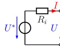
$$R_i = \frac{(R_2 + R_3) \cdot R_4}{(R_2 + R_3) + R_4} = \frac{(500 \Omega + 300 \Omega) \cdot 800 \Omega}{(500 \Omega + 300 \Omega) + 800 \Omega} = 400 \Omega$$
