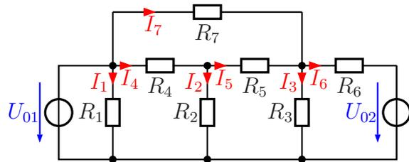
$$U_{01} = 12 \text{ V} \quad R_1 = 200 \, \Omega \quad R_3 = 1,5 \text{ k}\Omega \quad R_5 = 1,5 \text{ k}\Omega \quad R_7 = 3 \text{ k}\Omega$$
