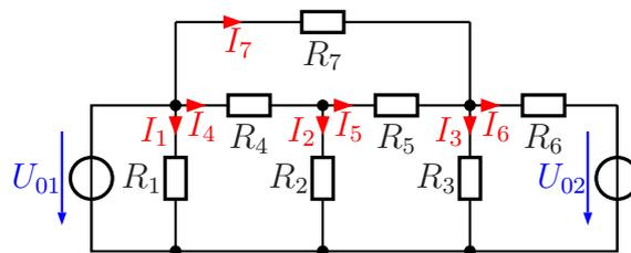
$$U_{01} = 12 \text{ V} \quad R_1 = 200 \, \Omega \quad R_3 = 1,5 \text{ k}\Omega \quad R_5 = 1,5 \text{ k}\Omega \quad R_7 = 3 \text{ k}\Omega$$
