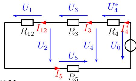
$$I_3 = I_{12} = I_5 = \frac{U_0}{R_4 + R_3 + R_{12} + R_5} = \frac{50 \text{ V}}{5 \text{ k}\Omega + 9,6 \text{ k}\Omega + 2,4 \text{ k}\Omega + 8 \text{ k}\Omega} = 2 \text{ mA}$$
