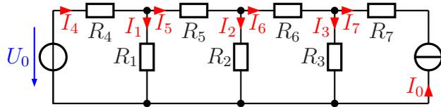
$$U_0 = 12 \text{ V} \quad I_0 = 20 \text{ mA} \quad R_1 = 1,4 \text{ k}\Omega \quad R_2 = 4 \text{ k}\Omega \quad R_3 = 1 \text{ k}\Omega$$
