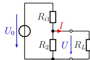
$$R_i^* = \frac{R_{i1} \cdot R_2}{R_{i1} + R_2} = \frac{100\ \Omega \cdot 400\ \Omega}{100\ \Omega + 400\ \Omega} = 80\ \Omega$$
