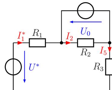
$$U^* = R_1 \cdot I_0 = 1 \text{ k}\Omega \cdot 10 \text{ mA} = 10 \text{ V}$$
