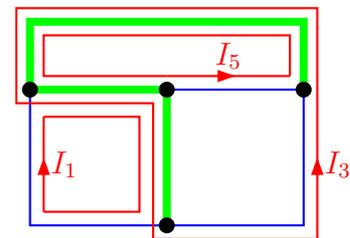
$$\begin{aligned} (1) \quad & (R_1 + R_4 + R_2) \cdot I_1 & + (R_4 + R_2) \cdot I_3 & + R_4 \cdot I_5 & = & U_{01} - U_{02} \\ (3) \quad & (R_4 + R_2) \cdot I_1 & + (R_4 + R_2 + R_3) \cdot I_3 & + R_4 \cdot I_5 & = & U_{03} - U_{02} - U_{04} \\ (5) \quad & R_4 \cdot I_1 & + R_4 \cdot I_3 & + (R_4 + R_5) \cdot I_5 & = & -U_{04} \end{aligned}$$
