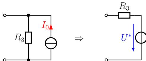
$$U^* = R_3 \cdot I_0 = 1 \text{ k}\Omega \cdot 20 \text{ mA} = 20 \text{ V}$$
