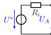
$$U^* = \frac{R_2}{R_1 + R_2} \cdot U_0 = \frac{400 \Omega}{100 \Omega + 400 \Omega} \cdot 15 \text{ V} = 12 \text{ V}$$
