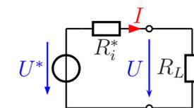
$$U = \frac{U^* \cdot R_L}{R_i^* + R_L} = \frac{9,6\ \text{V} \cdot 20\ \Omega}{80\ \Omega + 20\ \Omega} = 1,92\ \text{V}$$
