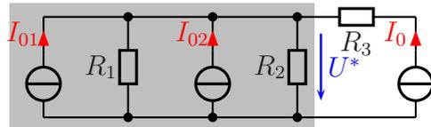
$$I_{01} = \frac{U_{01}}{R_1} = \frac{4 \text{ V}}{500 \Omega} = 8 \text{ mA}$$
