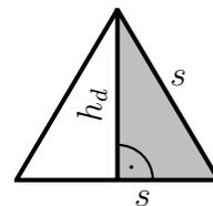
$$\begin{aligned} h_d^2 + \left(\frac{s}{2}\right)^2 &= s^2 \\ h_d^2 &= s^2 - \left(\frac{s}{2}\right)^2 \\ h_d^2 &= s^2 - \frac{1}{4}s^2 \\ h_d^2 &= \frac{3}{4}s^2 \\ h_d &= \sqrt{\frac{3}{4}s^2} \\ h_d &= \frac{\sqrt{3}}{2} \cdot s \end{aligned}$$
