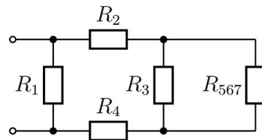
$$R_{567} = R_5 + R_{67} = 40 \Omega + 80 \Omega = 120 \Omega$$
