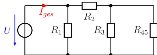
$$R_{45} = R_4 + R_5 = 700 \Omega + 800 \Omega = 1,5 \text{ k}\Omega$$
