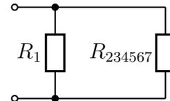
$$R_{234567} = R_2 + R_{3567} + R_4 = 190 \Omega + 48 \Omega + 62 \Omega = 300 \Omega$$
