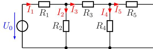
$$\begin{aligned} U_0 &= 12 \text{ V} \\ R_1 &= 4 \text{ k}\Omega \\ R_2 &= 1 \text{ k}\Omega \\ R_3 &= 3,1 \text{ k}\Omega \\ R_4 &= 9 \text{ k}\Omega \\ R_5 &= 1 \text{ k}\Omega \end{aligned}$$
